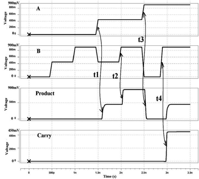
Fig. 14. Transient response of the ternary 1-bit multiplier.
