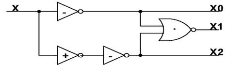
Fig. 9. Schematic diagram of ternary decoder.
