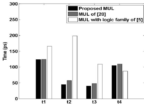
Fig. 15. Transient delay of CNTFET-based ternary multipliers.
