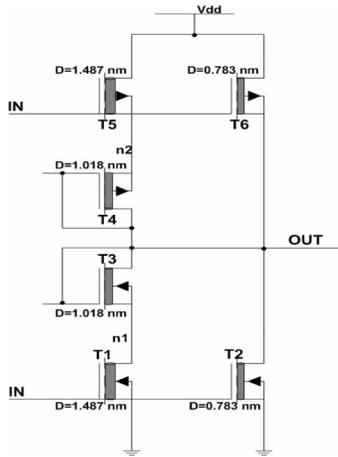
Fig. 4. Proposed CNTFET-based STI design.
