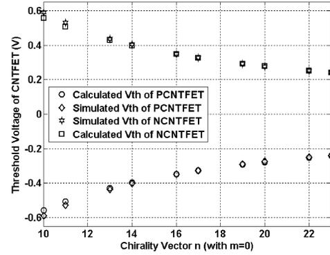
Fig. 2. Threshold voltage of CNTFETs versus  $n$  (for  $m = 0$ ).
