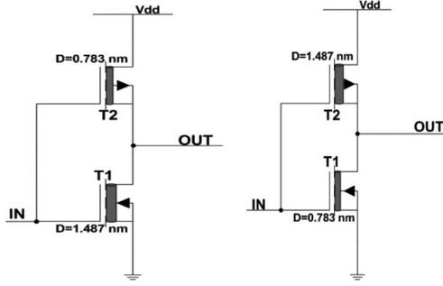
Fig. 6. Schematic diagram of (a) NTI and (b) PTI.
