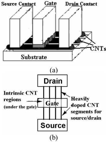
Fig. 1. Schematic diagram of a CNT transistor. (a) Cross sectional view. (b) Top view.
