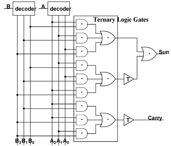
Fig. 10. Schematic diagram of ternary HA [20].
