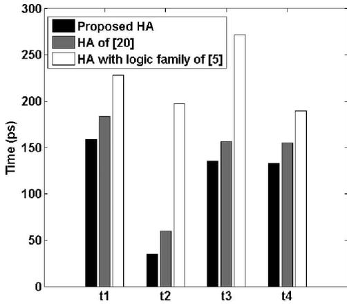
Fig. 13. Transient delay of CNTFET-based ternary HAs.
