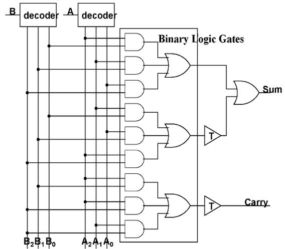
Fig. 11. Schematic diagram of proposed ternary HA.
