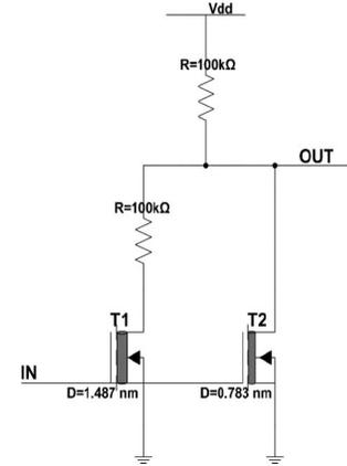
Fig. 3. Schematic diagram of CNTFET-based STI proposed in [5].
