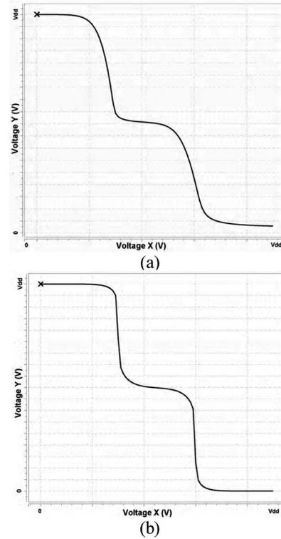
Fig. 5. VTC of STI. (a) STI in Fig. 3. (b) STI in Fig. 4.
